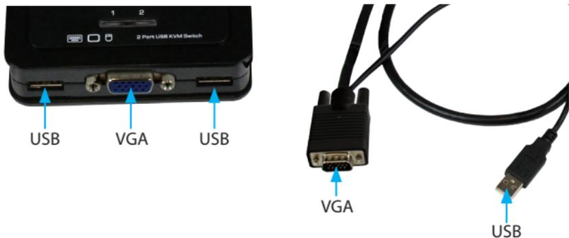
6. Connect the attached KVM cables to Computer 1.
