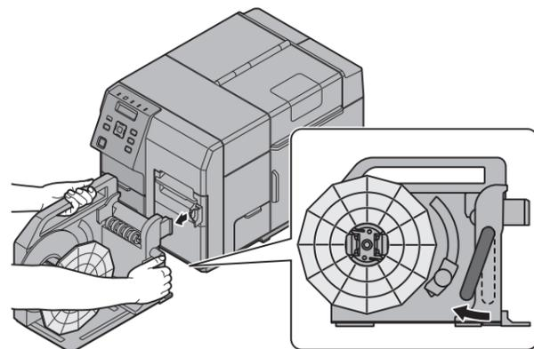
When media has finished rewinding, hold it by the core to pull it out.
