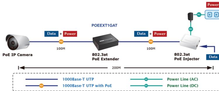
Refer to the diagram below for the maximum supported power output at each distance.
