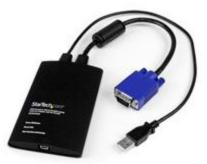
The NOTECONS02 Portable USB Crash Cart Adapter lets you turn your laptop into a portable console for rack servers, PCs, ATMs, kiosks and more, now with local file transfer built-in. Simply connect the crash cart adapter to your laptop using the included USB cable, then connect the integrated USB and VGA cables to your server for instant, BIOS-level control.
