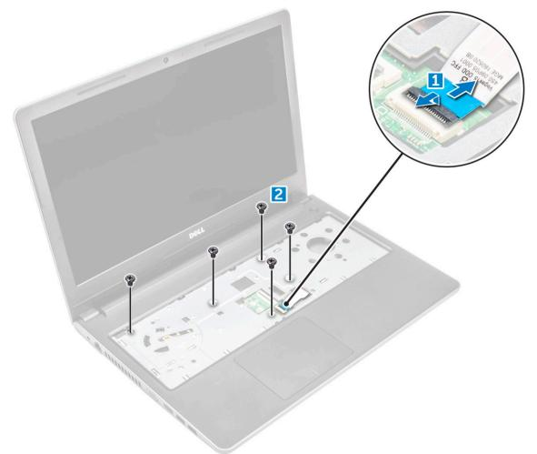
4 Flip the computer and remove the screws (8 screws - M2.5L8; 3 screws - M2L2; 2 screws- M2L2) that secure the base cover to the computer.
