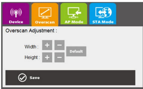
**Overscan:** Adjust the overall width and height of the streaming image to better fit on the remote display.
