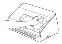
2 Open the Top Cover. Wipe the Control Panel with a dry, soft, and lint-free cloth to remove dust.
