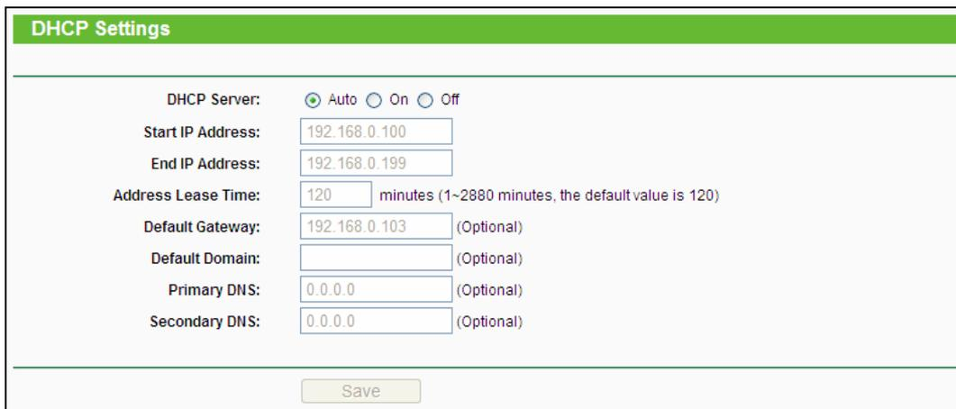
The screenshot shows the 'DHCP Settings' page with a green header. The 'DHCP Server' section has three radio buttons: 'Auto' (selected), 'On', and 'Off'. Below this are several input fields: 'Start IP Address' (192.168.0.100), 'End IP Address' (192.168.0.199), 'Address Lease Time' (120 minutes), 'Default Gateway' (192.168.0.103), 'Default Domain', 'Primary DNS' (0.0.0.0), and 'Secondary DNS' (0.0.0.0). A 'Save' button is at the bottom.
