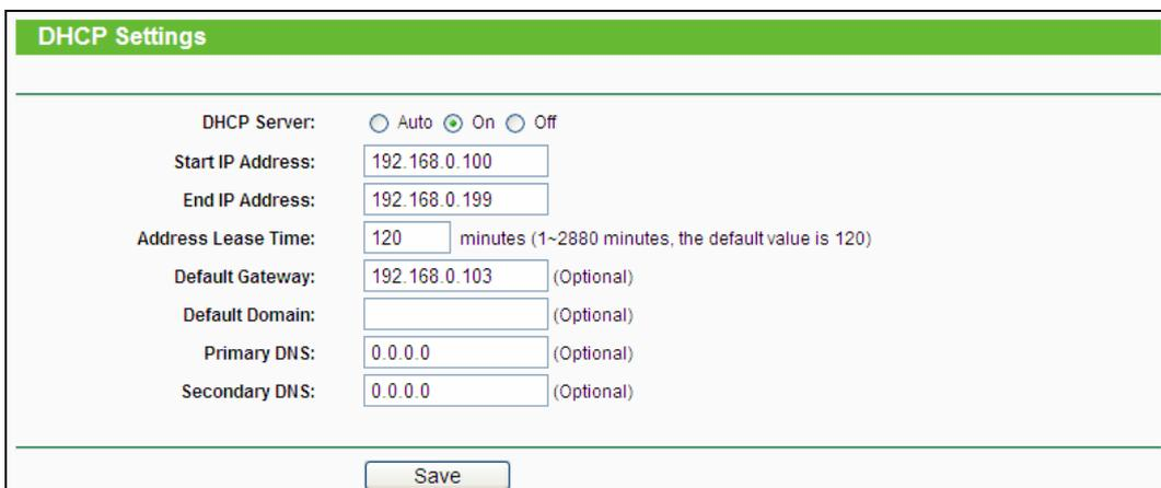
The screenshot shows the 'DHCP Settings' page with a green header. The 'DHCP Server' section has three radio buttons: 'Auto', 'On' (selected), and 'Off'. Below this are several input fields: 'Start IP Address' (192.168.0.100), 'End IP Address' (192.168.0.199), 'Address Lease Time' (120 minutes), 'Default Gateway' (192.168.0.103), 'Default Domain', 'Primary DNS' (0.0.0.0), and 'Secondary DNS' (0.0.0.0). A 'Save' button is at the bottom.
