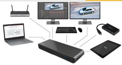
The dock features two Thunderbolt 3 USB-C ports for connecting to Thunderbolt devices and other peripherals that use the USB-C connector, as well as DisplayPort video output. For dual 4K video capability, you can use a 4K 60Hz capable video adapter to connect a second 4K 60Hz display to one of the dock's Thunderbolt 3 USB-C peripheral ports.
