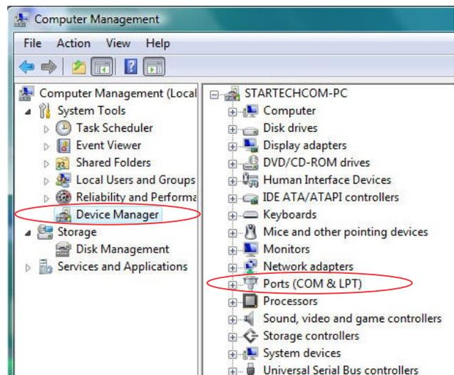
Double-click on the “Ports (COM & LPT)” option. The additional COM port should be visible.
