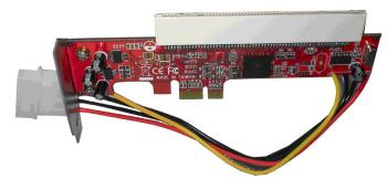
**Note**: If the spare PCIe bracket is used, the bracket on the PCI card must be removed. Full profile PCI cards may not fit in the system.
