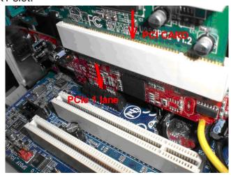
**Note**: PCIe slots are backwards compatible with smaller PCIe cards, so a x4 or greater slot can be used.
