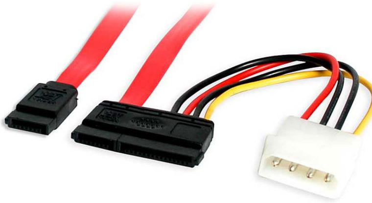
This SATA Data and Power Combo Cable features a combination 22-pin SATA female data and power connector as well as an LP4 power connector and female SATA data connector, allowing you create a conventional Serial ATA data connection to a computer while powering the drive through an LP4 connection to the computer power supply.
