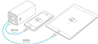
The 5V/2A USB port can automatically adjust its voltage to charge your 5V/1A devices.
