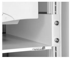
Deep Shelf - Before installing the deep shelf into the cabinet you must first join the mounting bracket to the shelf using the screws and nuts provided. Move the nuts in the cabinet to the desired hight and fasten the shelf's brackets to the front and rear posts.
