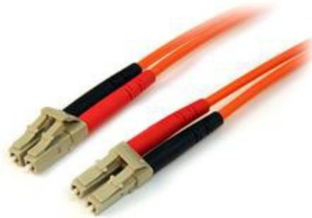
The 50FIBLCLC2 2-meter (6.6ft) Multimode 50/125 Duplex Fiber Patch Cable is terminated at both ends with LC (male) connectors to provide the necessary connection between fiber networking devices for high-speed, long distance networks.
