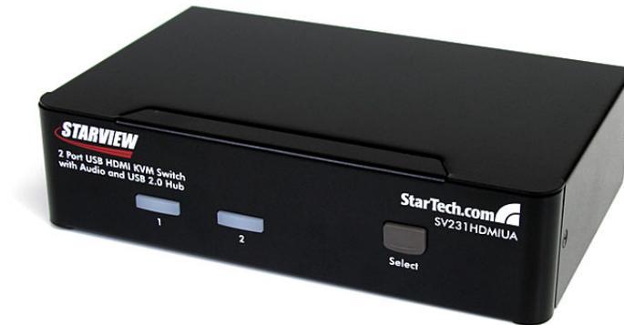
The SV231HDMIUA 2-port USB HDMI KVM Switch lets you control two USB-enabled multimedia computers or devices with HDMI video interfaces, using a single peripheral set/console (USB keyboard, mouse, monitor, speakers and microphone).
