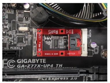
3. The SATA port on the adapter now functions as a standard SATA port to the specification of the motherboard's mSATA port.
