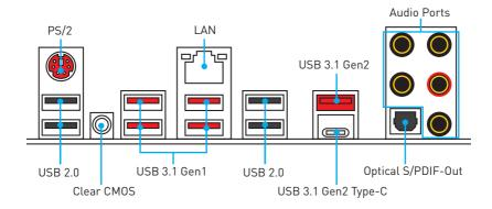
• Clear CMOS button - Power off your computer. Press and hold the Clear CMOS button for about 5-10 seconds to reset BIOS to default values.
