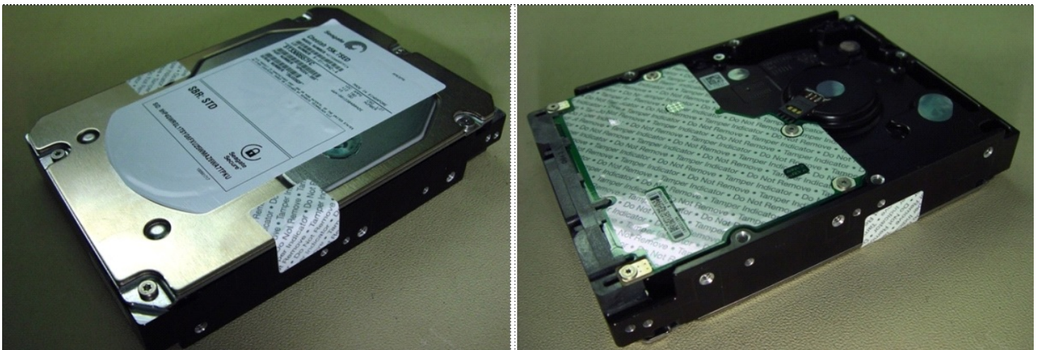
Figure 10. Example of FIPS tamper evidence labels.
