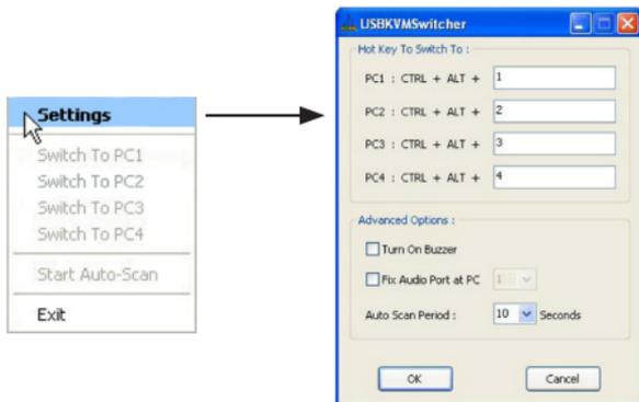
From within the KVM Switcher software, you also have the option to fix the audio/MIC channel to the selected PC. Once this option is checked, the audio/MIC channel will be fixed and become non-switchable without re-configuration.
