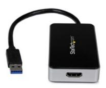
The USB32HDEH USB 3.0 to HDM® Adapter turns a USB 3.0 port into an HDMI output port with 1920x1200/1080p video support. The adapter features a built-in 1-Port USB 3.0 hub, which offers a connection port in place of the USB port used for connecting the HDMI adapter – an ideal workaround for Ultrabook™ or laptop users, where only a limited number of USB ports are available.
