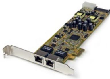
The ST2000PEXPSE Dual Port PoE NIC provides two 10/100/1000 Mbps PoE RJ45 ports that can provide up to 25.5W of power each, combining a network data connection and power on a single cable, for less clutter and convenient installations in remote locations.
