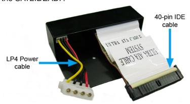
3. Connect the ribbon cable and power cable to the connectors on the IDE hard drive.
