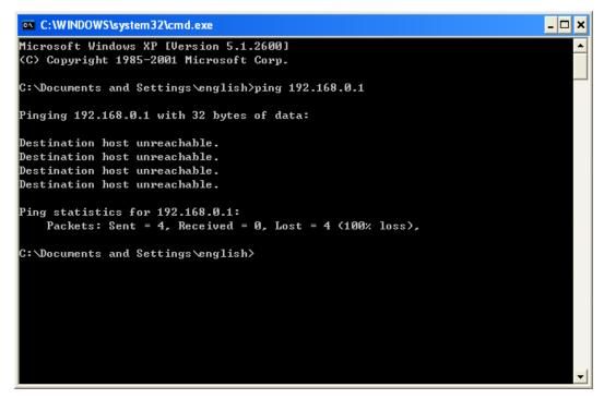
Figure 3-2 Failure result of Ping command
