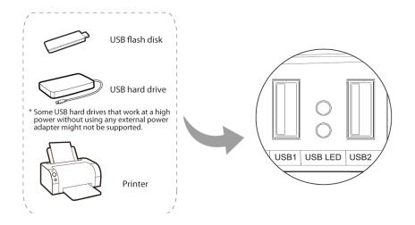
Figure 2-2 USB Installation
