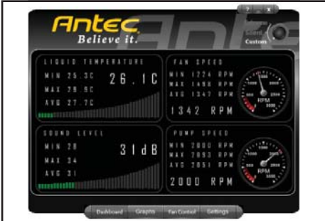
Included software provides essential tools to control and monitor the KÜHLER H 2 O 920
