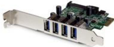
The PEXUSB3S4V PCI Express USB 3.0 Card (with SATA Power) adds 4 external USB 3.0 ports to any PCI Express-enabled computer system. SuperSpeed USB 3.0 provides up to 5 Gbps of data bandwidth, while remaining backward compatible with existing USB 2.0 devices at 480Mbps.
