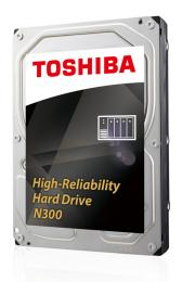
Toshiba's N300 3.5-inch internal hard disk offers unprecedented reliability for NAS and other high-performance storage systems. It is optimized to meet the reliability, endurance, performance and scalability requirements of 24-hour x 7-day high-capacity storage for personal, home office and small business use. The N300 is available in capacities of up to 6 TB.
