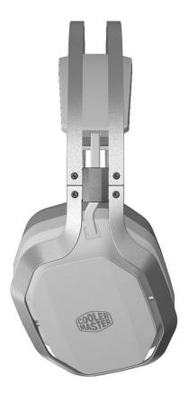
Side view with closed Bass FX covers (Bass FX OFF) for a increased treble and passive noise isolation
