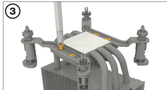
Fasten the Intel push-pins (3) mounting on the cooler. You can use any cross-tip screwdriver for this.
