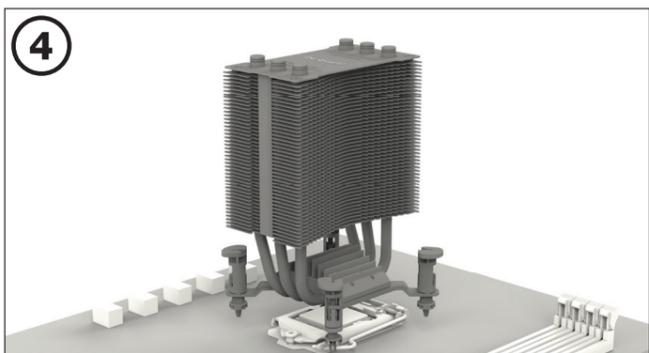
Place the cooler onto the CPU unit.
