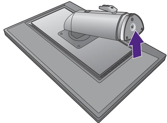
Orient and align the stand base socket with the end of the stand arm, then push them together. Tighten the thumbscrew on the bottom of the monitor base as illustrated.
