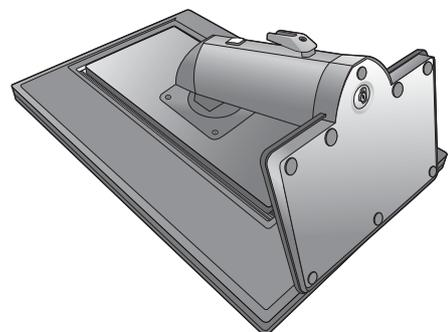
Extend the stand to the maximum extended position. And rotate the monitor 90 degrees counterclockwise as illustrated.
