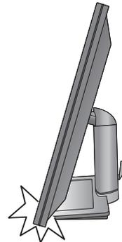
To extend the monitor stand to a higher position, press the lower part of the height release on the stand while holding the bottom of the monitor at the same time. And pull the stand and the monitor upward together to the desired height.
