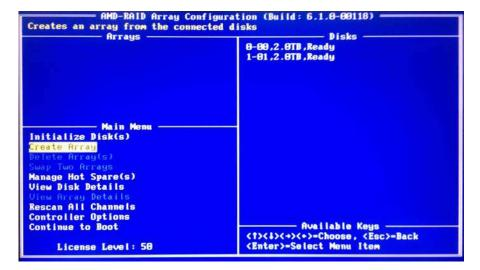
Use the arrow keys to select the hard drives to be included in the RAID array and press <Ins>. The selected hard drives will be shown in green. To use all of the hard drives, simply press <A> to select all. Then press <Enter>.
