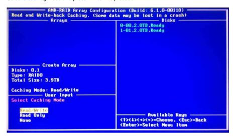
Press <C> to confirm and then press <Esc> to return to the previous screen.
