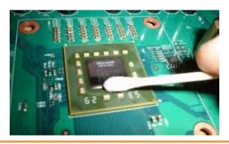
3. APPLYING THERMAL COMPOUND. Apply thermal compound: lightly coat the *Intel X99 PCH* (SB) with <u>electrically non-conductive</u> thermal grease - for example Arctic Cooling MX-2  $^{\text{TM}}$ , MX-4  $^{\text{TM}}$  or GELID GC-Extreme  $^{\text{TM}}$ . EKWB recommends to apply the thermal grease in cross form for the best performance (see sample picture).
