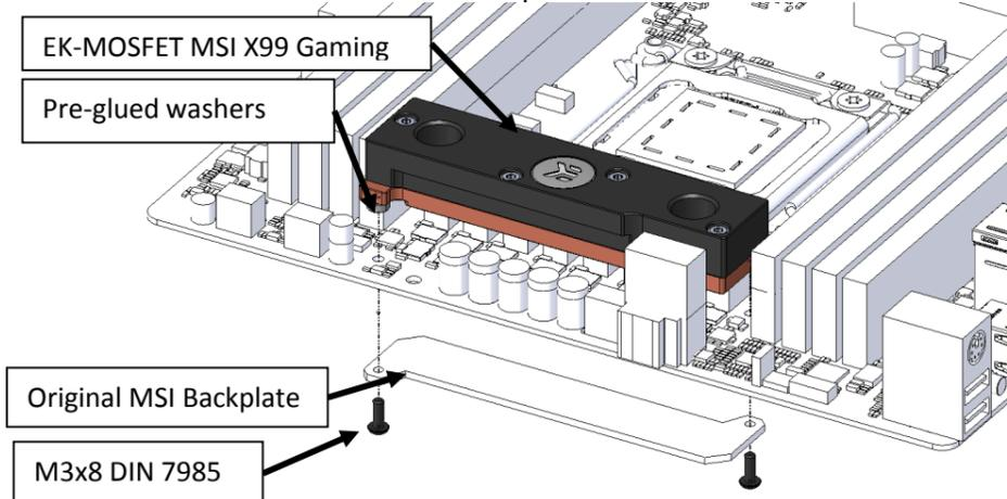
**ATTACHING WATERBLOCK/BACKPLATE ON MOTHERBOARD.** When waterblock is safely placed on motherboard, please align the openings and fasten the waterblock to dbackplate using the enclosed M3x8 DIN7985 screws to the motherboard's circuit board. It is recommended that you check for unwanted contacts before powering up the system.
