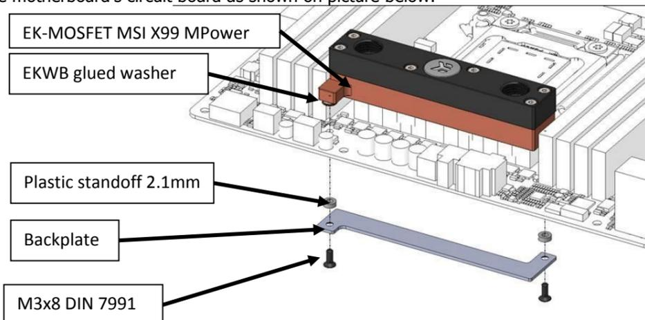
**ATTACHING WATERBLOCK/BACKPLATE ON MOTHERBOARD.** When waterblock is safely placed on motherboard, please align the openings and fasten the waterblock to dbackplate using the enclosed M3x10 DIN7991 screws to the motherboard's circuit board. It is recommended that you check for unwanted contacts before powering up the system.
