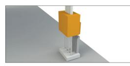
Position the cooler above the CPU, passing the attached AMD mounting brackets (5) over the projecting M3x15 screws (9)
