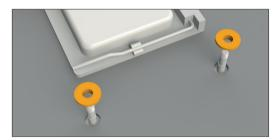
Now fasten the backplate on the front side of the motherboard using the C-profile spacers (12) by pressing these onto the notches in the M3x15 screws (9) until they click in.
