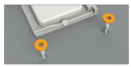
Now fasten the backplate using the C-profile spacers (12) by pressing these onto the notches in the AM4 M3x15 screws (10) until they click in.
