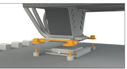
and affix by turning the AM4 M3x15 screws (10) from the rear
