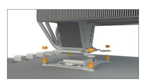
Place the hexagonal nuts (8) over the LGA 2011(-3) square ILM spacer nuts (7) and progressively tighten these in a crosswise manner until firm using the hexagonal wrench (14).
