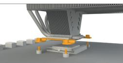
and affix by turning the M3x15 screws (9) from the rear side of the motherboard.
