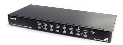
This 16 Port USB KVM Switch offers a dependable computer management tool that allows you to control up to 16 USB connected computers from one keyboard, mouse and monitor.
