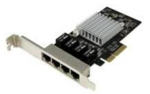
Here's a dependable and cost-effective way to add four high-performance Gigabit Ethernet ports to your server or desktop computer, through one PCI Express slot.
