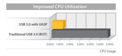
Testing results were obtained using an Intel® lvy Bridge system, a UASP-enabled StarTech.com Enclosure, and a SATA III solid state drive.
