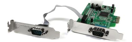
The PEX2S553LP low profile/half-height PCI Express Serial Card turns a PCI Express slot into two RS232 (DB9) serial connections.
