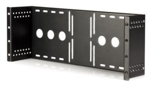
This 19in LCD mounting bracket lets you mount almost any retail LCD or Touch screen panel into a server/storage rack/cabinet. The LCD mounting bracket is designed to support 100mm and 75mm VESA mounted LCD panels, and meets ANSI/EIA RS-310-D standards rack mounting; the bracket features a unique adjustable design that enables an LCD panel to be mounted into the cabinet at various depths - allowing the rack/cabinet door to be closed, ensuring optimal server/equipment storage.
