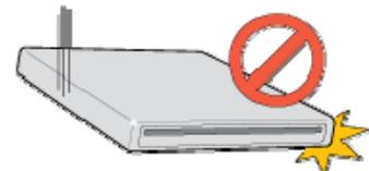
Do not move the drive while in operation. Do not attempt to open the disc tray by force. Make sure that you close all open applications before you open the tray. Always use the Eject button to open and close the tray.
