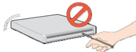
Do not insert a pin into the emergency hole while the drive is in operation. Keep your hand away from the tray while the drive is in operation. This can result in damage to the product or human body.
