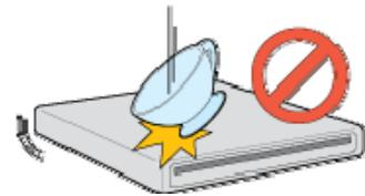
Do not drop the drive. Protect the drive from severe shocks.
