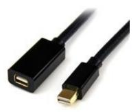
The MDPEXT3 3ft Mini DisplayPort 1.2 Extension Cable features one Mini DP male connector and one Mini DP female connector, extending the connection between your Mini DisplayPort devices by up to 3ft.
