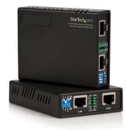
The 110VDSLEXTGB VDSL Ethernet extender kit allows you to span a 10/100 network over extremely long distances (up to 1km) while still maintaining high-speed network connectivity. The device allows you to run the connection over standard RJ45 cabling, existing RJ11 phone lines, or any other set of single pair wires. The VDSL (VDSL2) kit is simple to install and provides an out-of-the-box solution as both the Ethernet-VDSL extender and receiver units are included.
